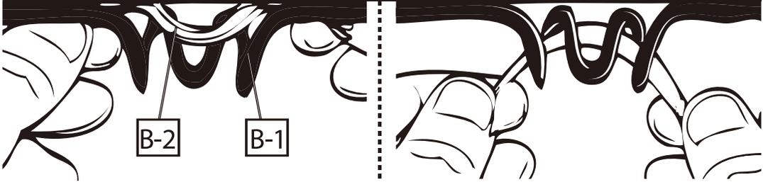
Find loops at top edge of net (B-2). Hook one loop over and around center of rim hook (B-1). Pull loop down to secure loop within rim hook. Repeat for remaining net loops.
