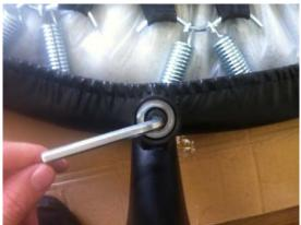
**Step 5**Place cap over tightened end and bang into place with a hammer (Photo 8 & 9)
