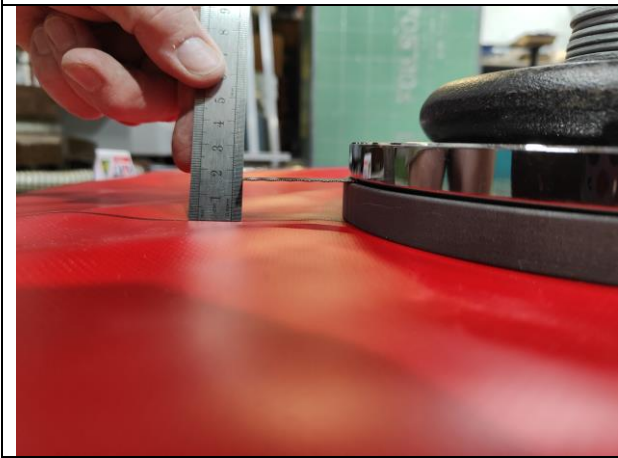
Photo 2: Depicts the feeler arm 16mm above the surface Passing
